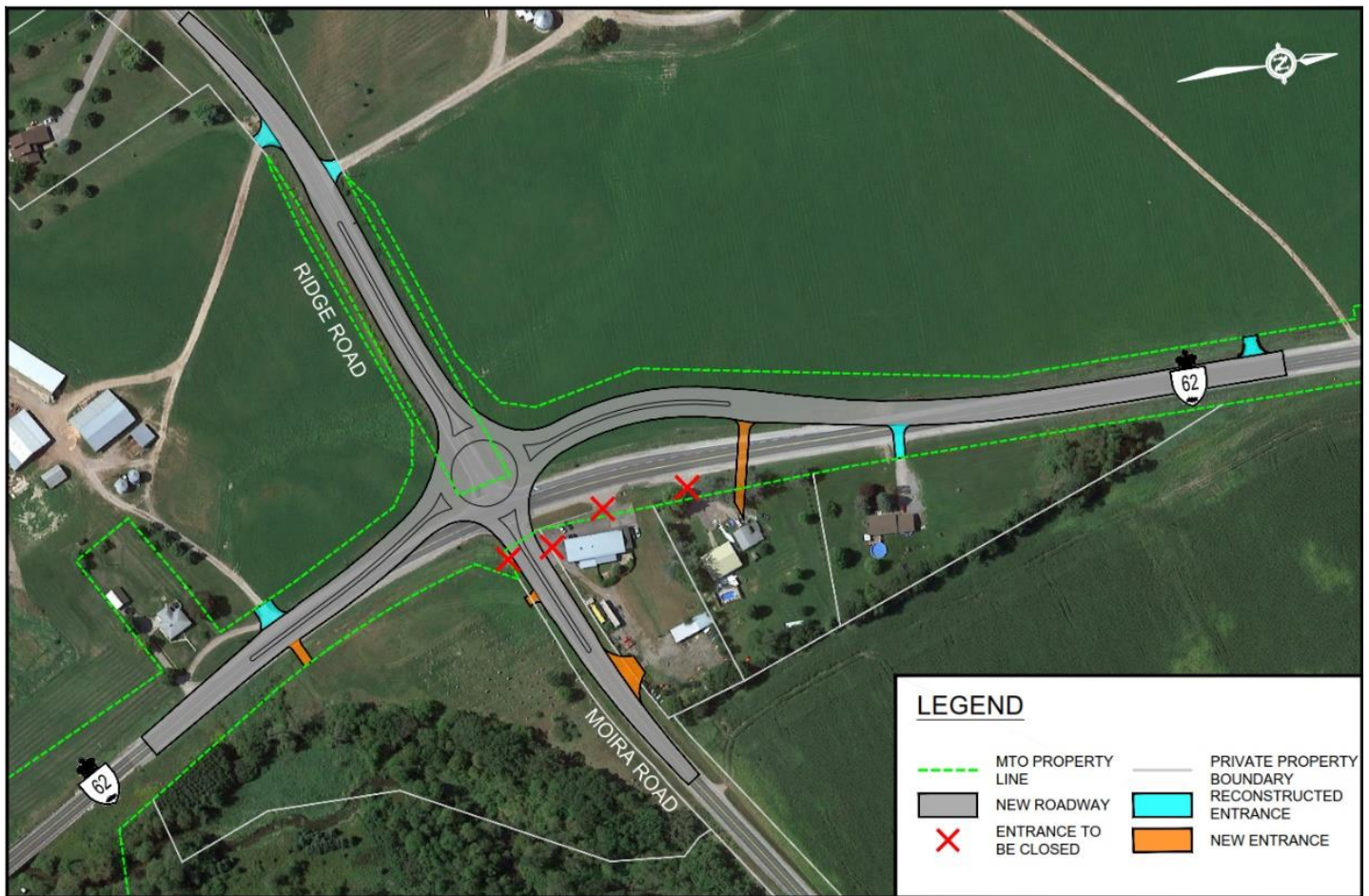
Figure 4: Intersection of Highway 62 and Moira/Ridge Road Property Entrance Impacts
